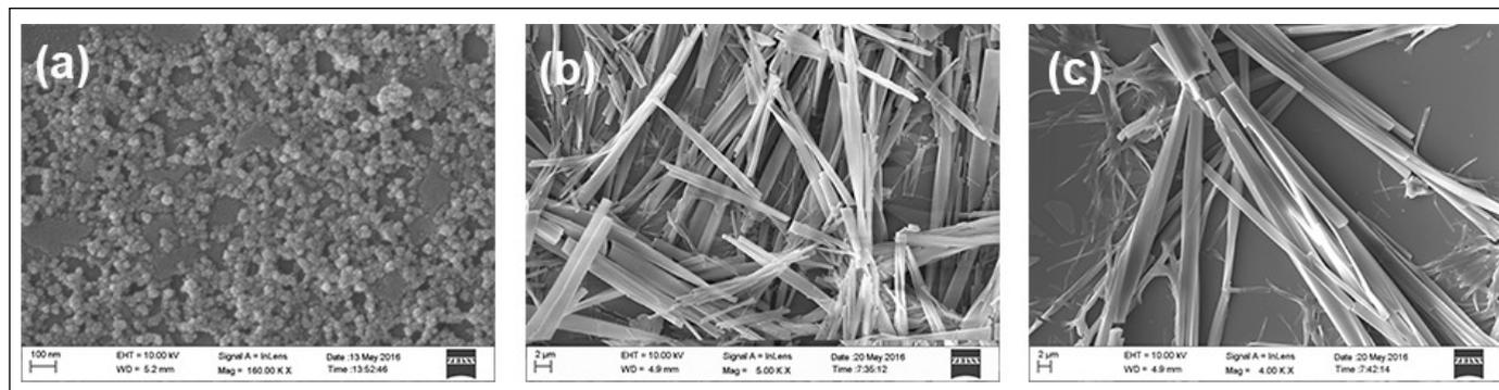
Figure 3 Self-assembly of TTBT in different solvent environments:(a) the aqueous dispersion of nanoparticles obtained by the reprecipitation method, (b) 1D nanorods in THF/water mixture and (c) 1D nanorods in THF/MeOH mixture.
